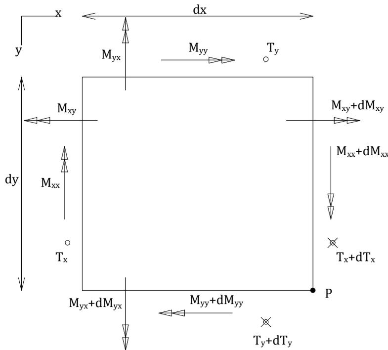
Figure 5: Plan view of the signs of the generalized stresses applied on an elementary part of the plate
