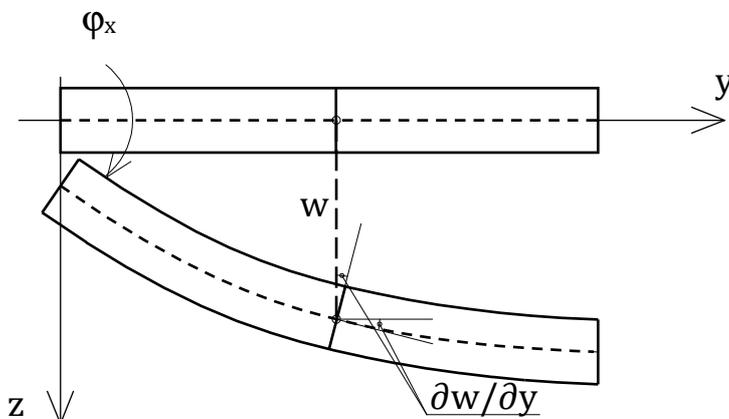
Figure 3: Displacement representation in the x-z plane
