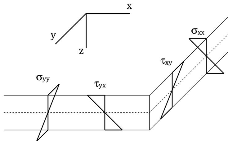
Figure 4: Point stresses on the positive face of a segmental plate element
