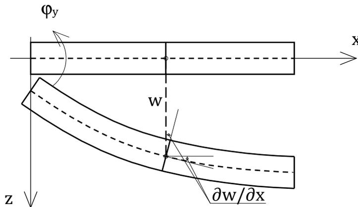
Figure 2: Displacement representation in the x-z plane
